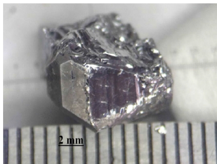
Figure 1 The picture of the single crystal sample with x = 0.3 prepared by the Sn-flux method according to the formula of Zn 4.4 Sb 3 Sn 3 In x ( x = 0-0.5 ).
