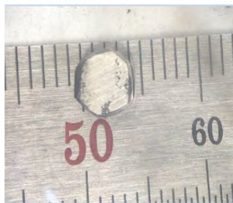
Figure 2 Single-crystal sample of type-I \text{Ba}_8\text{Ga}_{16-x}\text{Cu}_x\text{Sn}_{30} with x = 1 , grown with soaking temperature of 833 k.
